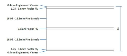
Fig.1 - Cross section through Stredor 44 ply faced door blank design
