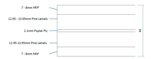
Fig.2 - Cross section through Stredor 44 MDF faced door blank design
