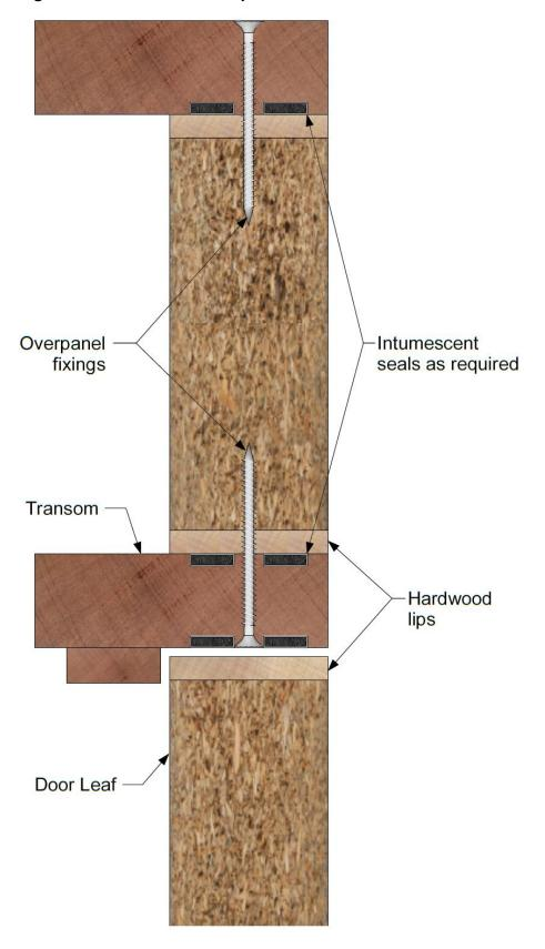
Figure 8.2 – Transomed overpanel – front elevation
