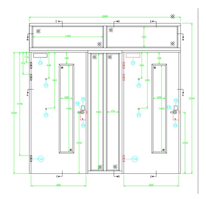
The following drawing is taken from test report WF 411193 and shows a modular fanlight above a door leaf. The components are given in the key underneath the drawing:
