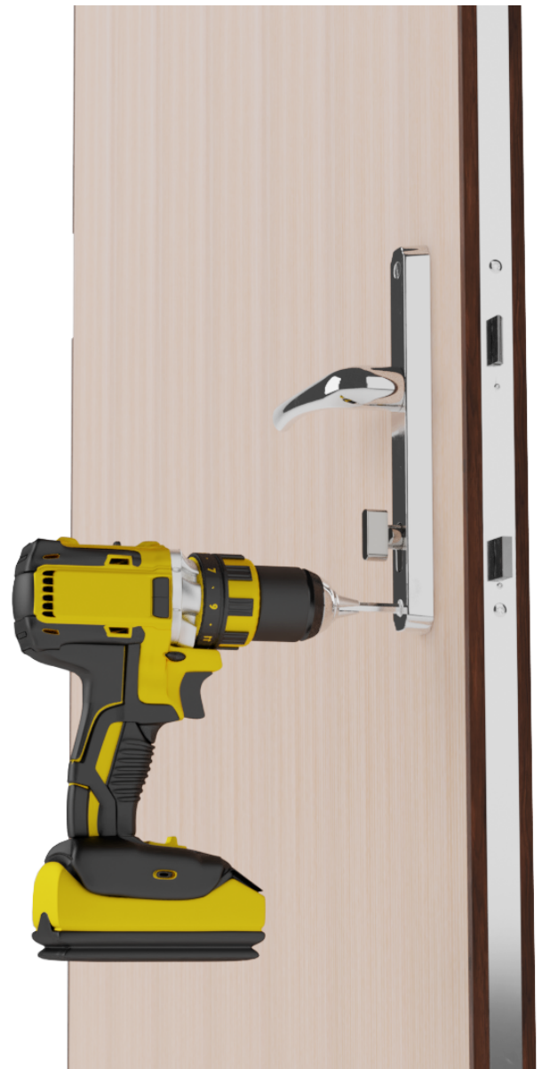
Handle being fitted to the leaf
