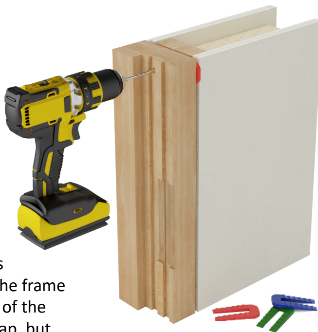
Pilot-drilling the frame to opening fixing with packer fitted
