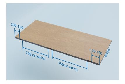
It is permitted to move the intermediate hinge, but the distance between the top hinge and intermediate hinge **or** the intermediate hinge and the bottom hinge must remain as tested. If either of these distances cannot be maintained it is permitted to add an additional hinge so that the maximum distance between hinges is not increased.
