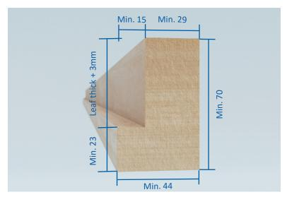
Cut frame components to the correct length, and prepare a 12mm trench joint.
