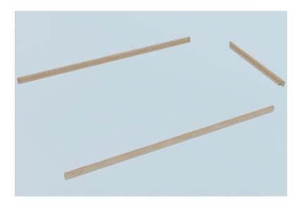
The frame must be a minimum of 70mm deep x 44mm thick, including a 15mm thick rebated stop. The frame should not overhang the wall on either side.
