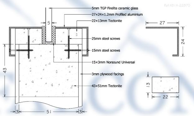
Figure 9 - Glazing system option 5 assembly and components
