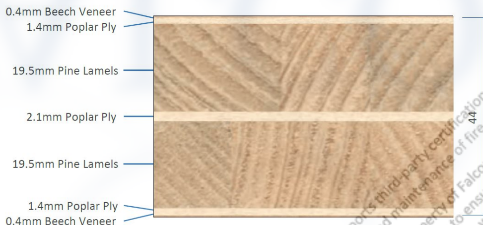
Fig. 4 – Cross section through Type B door blank design
