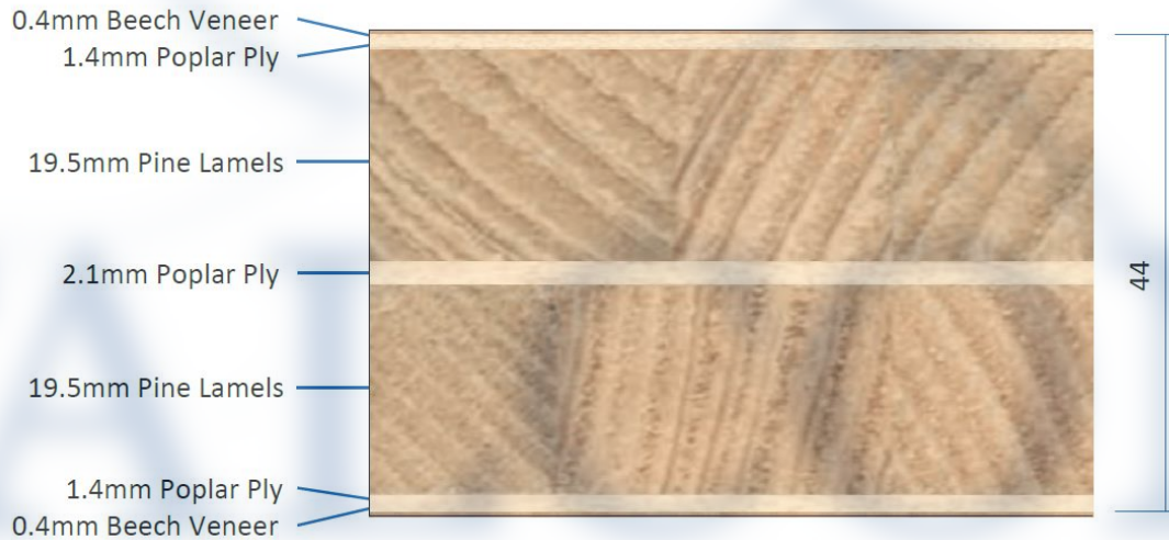
Fig.2 – Cross section through Type B door blank design
