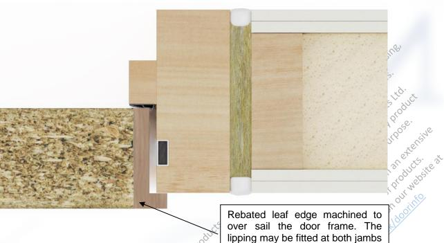
Fig. 5 – Over rebated edge detail
