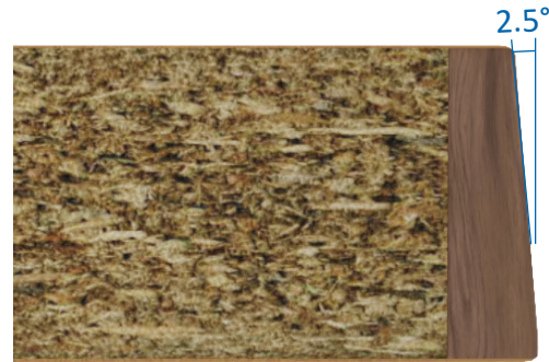
Maximum 2.5° chamfer to the leading edge
