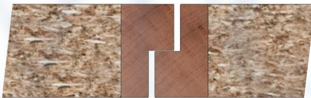
Equal Rebated | 20-25mm overall with 12-13mm deep equal rebate to be used at junction between head of leaves and flush overpanel or at the meeting edges of double doorsets without overpanels
