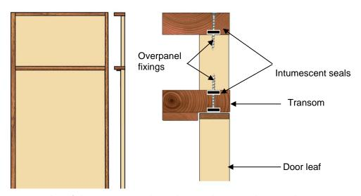
**Note:** Drawing is representative of doorset construction only; actual construction must be as the text within this document specifies.
