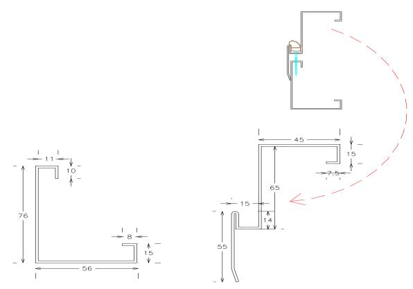
Plasterboard, mineral fibre, glass fibre and ceramic wool must not be used to backfill steel door frames. Appendix E details the leaf size ranges and intumescent seal specifications for steel frame constructions.
