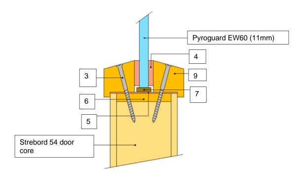
Therm-A-Glaze 60 System with Pyroguard EW60 (11mm)
