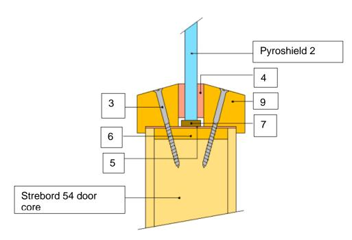
Therm-A-Glaze 60 System with Pyroshield 2
