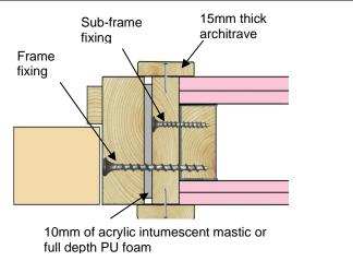
Guidance for various methods of sealing the frame to structural opening gap is also given in BS 8214: 2016, "Timber based fire door assemblies – code of practice" which may be referred to where appropriate.
