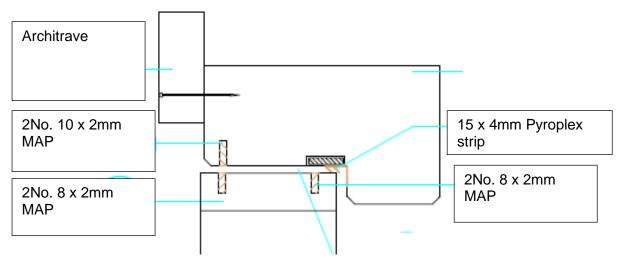
Figure to show positioning of intumescent seals when fitting the approved multi-point lock
