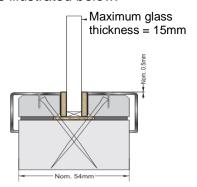
The Norsound Universal 60T glazing system has the following scope of application in addition to that described in sections 7.1 - 7.3. The Norsound Universal 60T is illustrated below:
