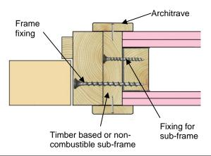
5. Timber based or non-combustible sub-frame up to 50mm thick, with gaps up to 10mm between the components filled on both sides with 10mm depth of acrylic intumescent mastic or full depth expanding PU foam, fire tested for this application to BS 476: Part 22: 1987 or BS EN 1634-1. Joint must be fitted with 15mm thick architraves overlapping at least 15mm each side.
