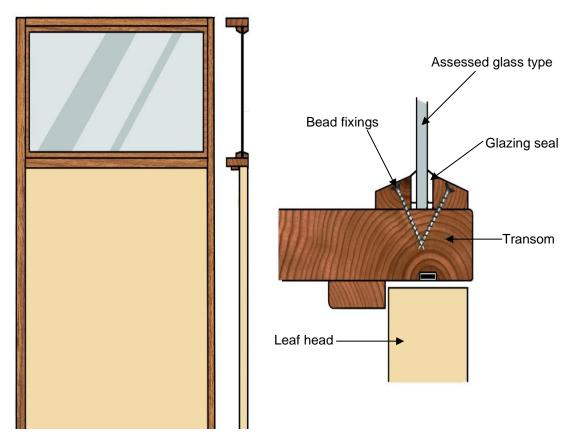
**Note:** Drawing is representative of doorset construction only; actual construction must be as the text within this document specifies.
