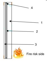
The vision panel is retained within the door leaf with either timber or steel beads, which must meet the specifications below:
