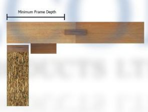
Head/jamb Mortice and tenon, or half-lapped joint, head twice screwed to each jamb joint or mitred joint which is glued with a non-thermally softening adhesive and the head twice screwed to each jamb.
