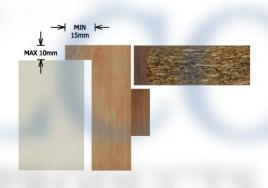
Transom members When a transom is used between a door and an overpanel, in single acting door assemblies the member shall be at least 70 x 32mm, and shall include minimum 12mm thick door stops on both sides (i.e. making a minimum 70 x 56mm thick overall section). In double acting door assemblies, the transom shall be at least 70 x 44mm. The transom must be fixed to the jambs with a mortice and tenon, or half-lapped joint. The overpanel must always be on the same plane as the door(s) below.
