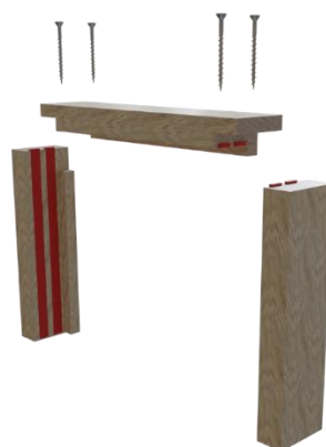
Trenched or Half Lapped Joint
