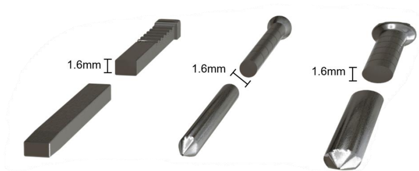
Figure 6.1 – Round, Oval & Rectangular pin detail – minimum dimension 1.6mm
