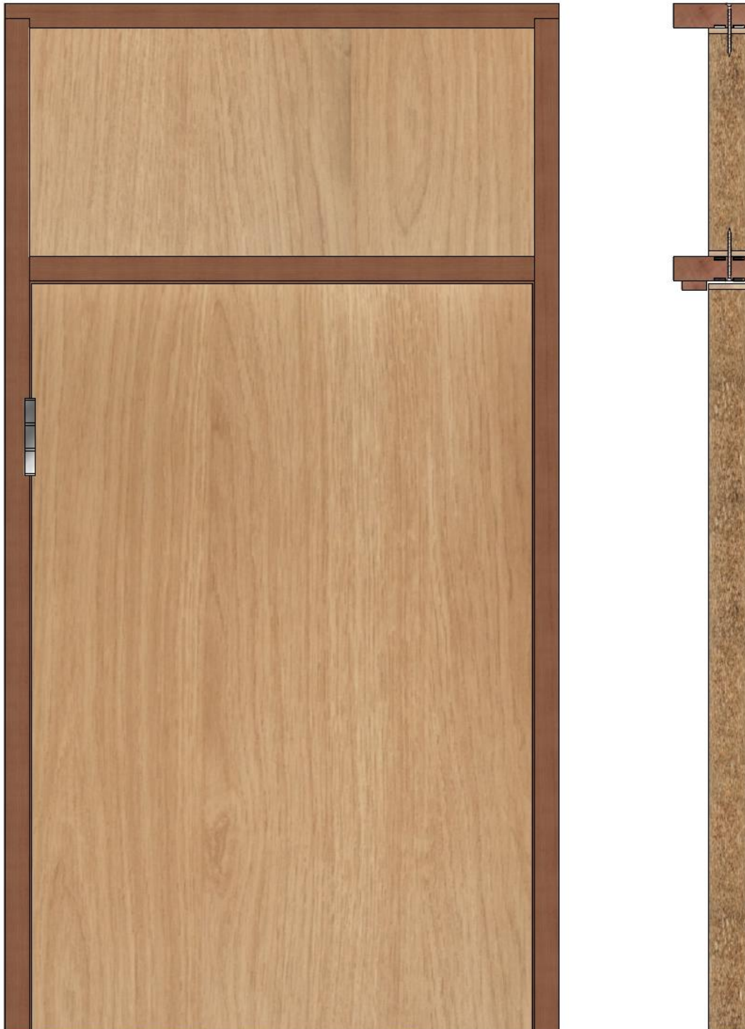
Figure 8.2 – Transomed overpanel – front elevation
