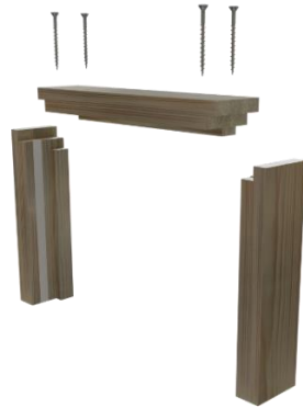
Half Lapped Joint
