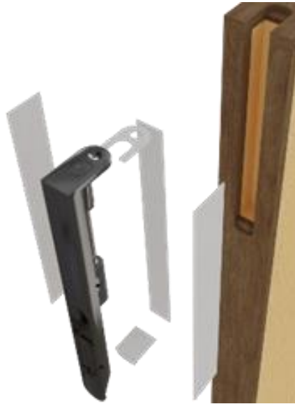
Figure 9 – Flush bolt installation and indicative intumescent protection
