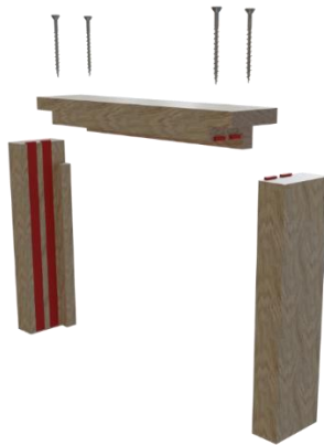
Trenched or Half Lapped Joint
