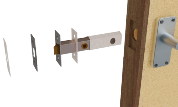
Example of lock & latch protection detail
