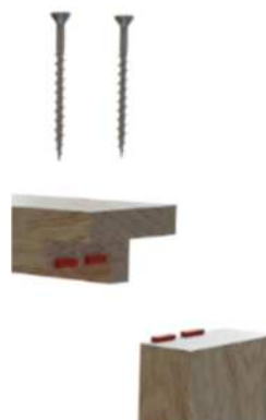
Trenched or Half Lapped Joint
