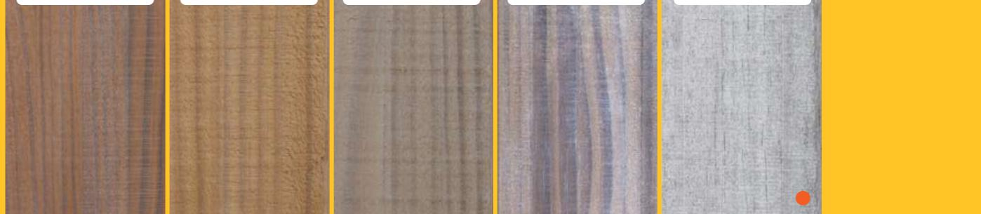
Colour may change/fade as a part of the natural weathering process. Coating performance on brushed finish may be lower compared with bandsawn finish.
