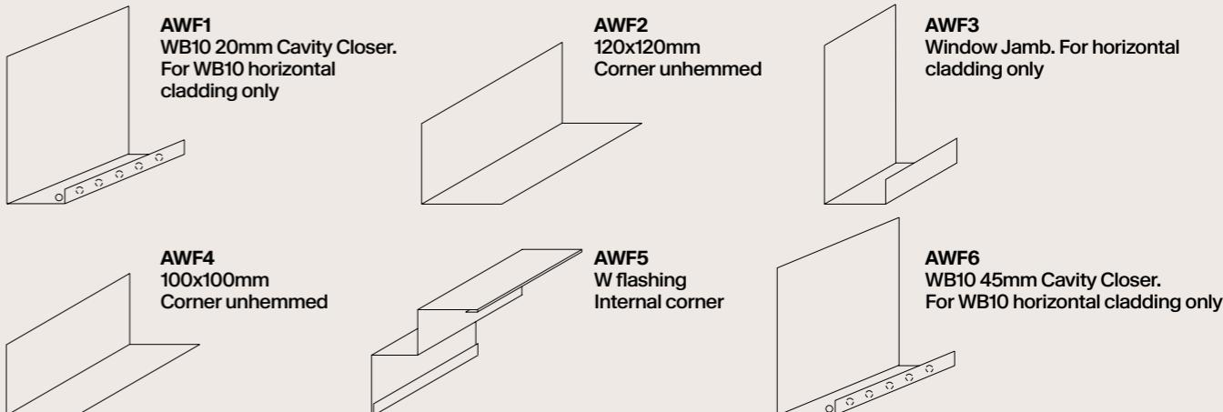
Supplied as 3m length stainless steel. Alternative flashings such as PVC may be used in conformance with E2 and Abodo details.
