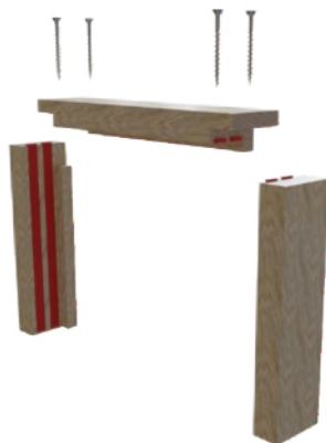
Trenched or Half Lapped Joint
